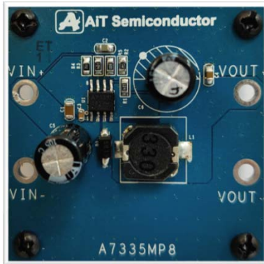
A7335 30V, 133kHz, 3.5A DC-DC Step-Down
