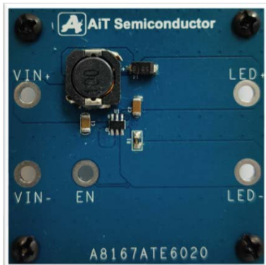
A8167A 1.2A, V_{REF}=200mV LED Driver IC
