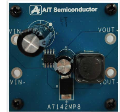
A7142 45V, 150kHz, 2A Simple Switcher Power Converter
